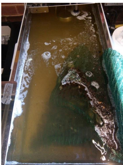
Figure 10 Inside the water bath on day two – ‘dirty’ water treatment. The green net holds the daffodil bulbs. The white foam residue is from dissolving of Cidox 300 tablets.
